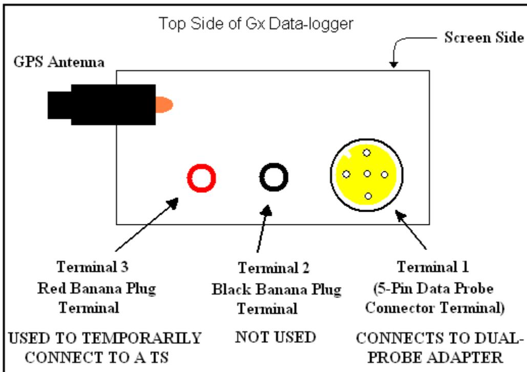
The red banana plug jack on the Gx is used to temporarily connect a test lead from the Gx to a pipe connection in order to record pipe-to-soil potentials for IR drop determination by the software (see Section II).
