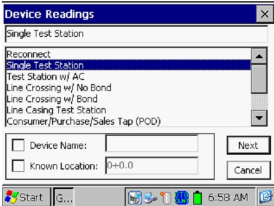
As can be seen from the above screen, you can choose from a number of “Devices”. In this case, you would tap on “**Single Test Station**” to highlight this selection.
