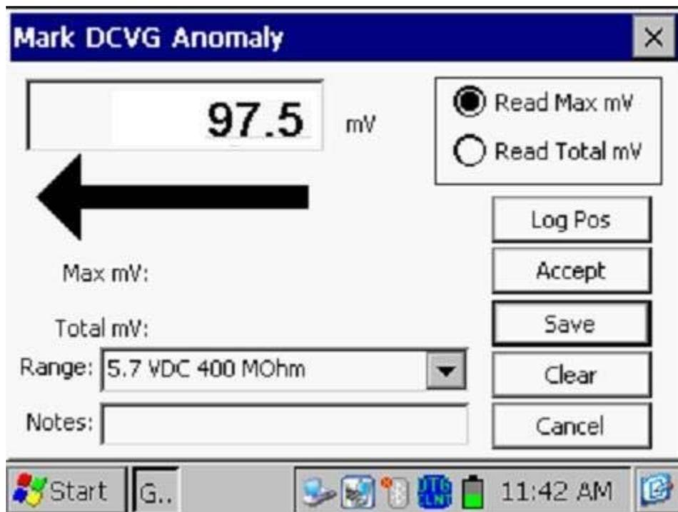
If you selected automatic logging of GPS position data at Sidedrains/Anomalies during the survey setup process (see Section III), the Gx data-logger will log the GPS data for the DCVG anomaly site when you “accept” the first side drain reading (see below). If you did not select this option during survey setup, you should tap on the “Log Pos” button if you would like to have GPS data logged for the anomaly location.
