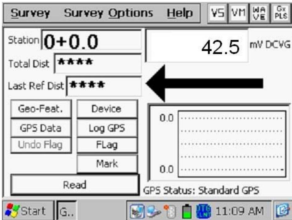
In the above “active” DCVG survey screen, the direction of the arrow (pointing to the left or pointing to the right) depends on the polarity of the DCVG voltage being measured. In the above case, the voltage being measured was positive which produced an arrow pointing to the left. The opposite would be true if the DCVG voltage reading had been negative (i.e., the arrow would point to the right).
