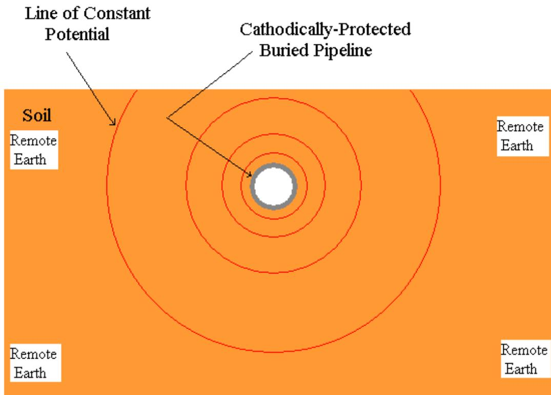
**Figure 1: Potential Gradient Associated with a Cathodically-Protected Pipeline (Equipotential Lines are closer together near the pipe, indicating that the potential drops quickly (initially) with distance away from the pipe).**
