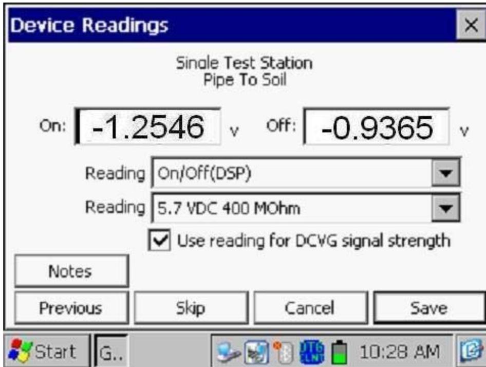
The On and Off pipe-to-soil potentials measured (per cycle) at the starting test station will be displayed on the above screen, assuming that one of the On/Off pairs voltmeter reading modes has been selected (see the “Reading” field on the screen).
