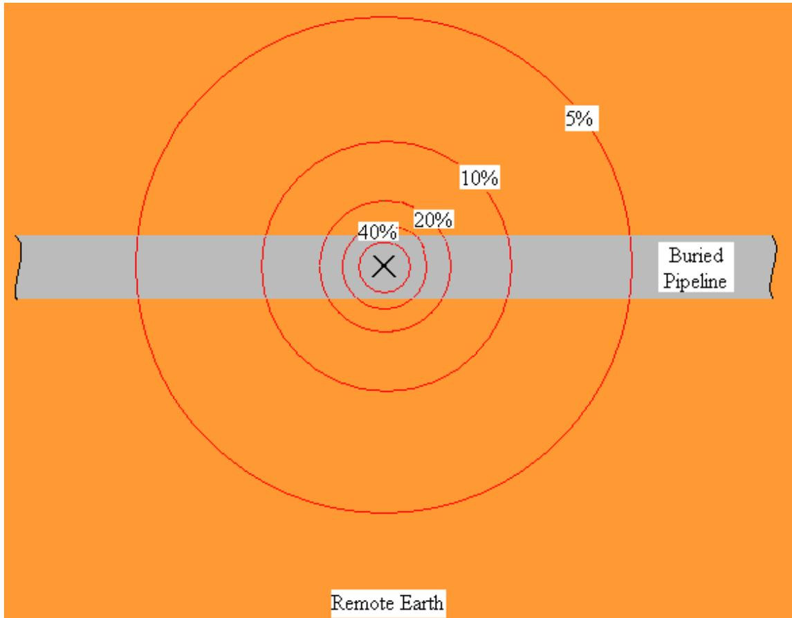
**Figure 3: Potential (Voltage) Gradient at the Surface of the Ground associated with a Coating Defect on a Buried Pipeline (concentric circles represent constant potential lines). The “X” symbol represents location of coating defect.**
