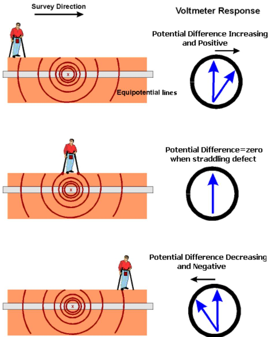
**Figure 7: In-Line DCVG Survey Technique**
