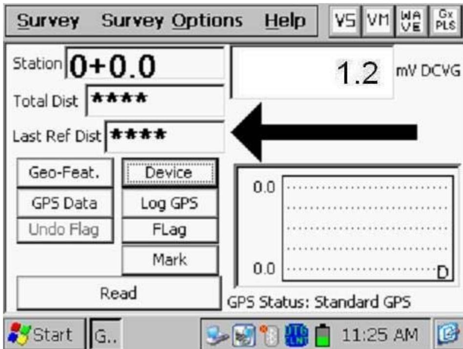
*Note:* The arrow on the Survey screen indicates the polarity of the DCVG voltage reading. For positive values, the arrow points to the left and for negative values, the arrow points to the right. This behavior is utilized to locate anomalies using the in-line approach (see Figure 7 in Section II.10).
