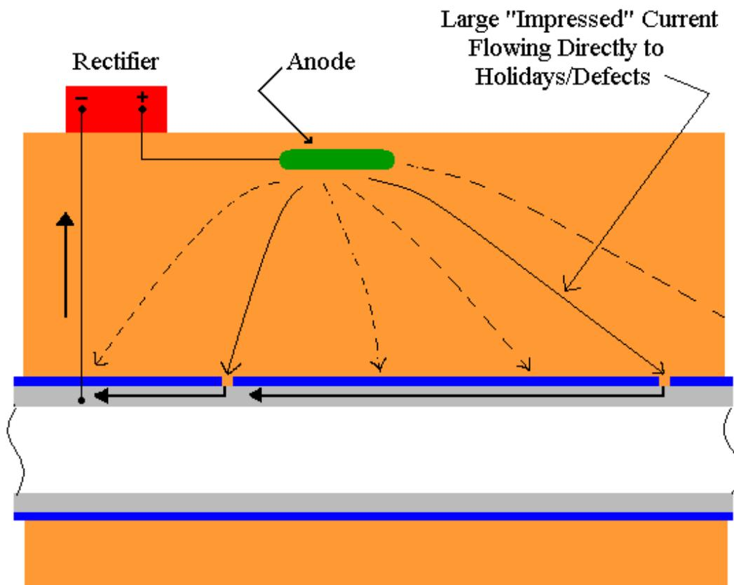
**Figure 2: The Influence of Coating Defects on Impressed-Current Flow Distribution along a Pipeline (locally high potentials occur at defect locations due to locally large currents flowing to the defects).**
