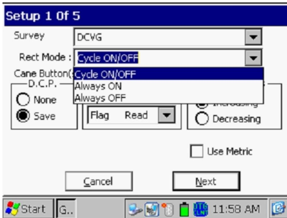
As can be seen from the above screen, there are 3 choices for “Rectifier Mode”. However, only the “Cycle On/Off” option should be selected for DCVG surveys, as rectifier current interruption is a requirement for this survey type.
